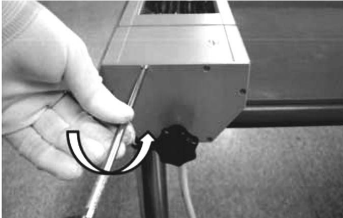
3 Remove 4 Phillips screws that hold connection box to heater:
