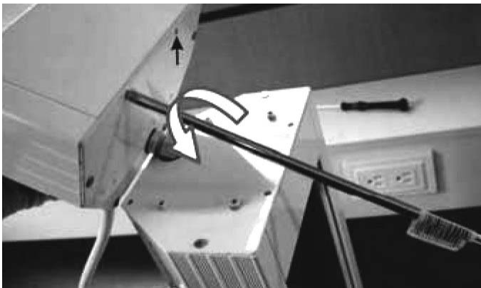
5 Slide the connection box front face plate out from the electrical connection box:
