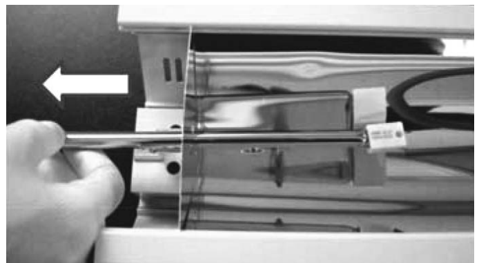
13 The heat lamp is fragile! Carefully slide old heat lamp out of heater through rectangular slot in end of reflector:
