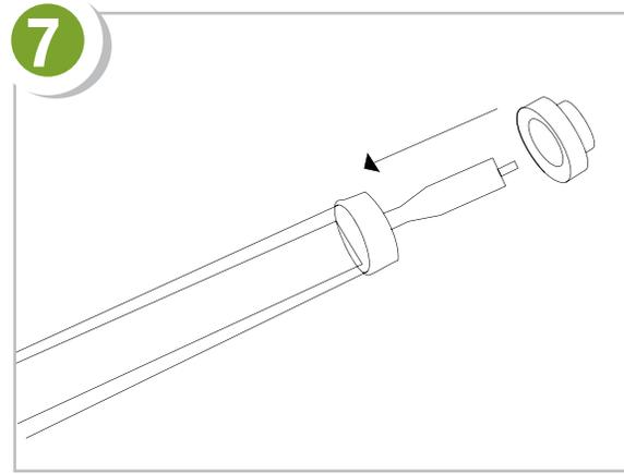
Place the safety rubber ring on top of the glass metal connection. **7** Rotate constantly the s-power high performance heat-pipe tube while inserting into the hole in the collector casing. **8** Insert the tube so the safety rubber of the heatpipe tube touches the end of the collector casing and then retrieve the tube out of the collector casing for 5mm. **9** Stiebel Eltron S-Power high performance heat pipe is now sealed.
