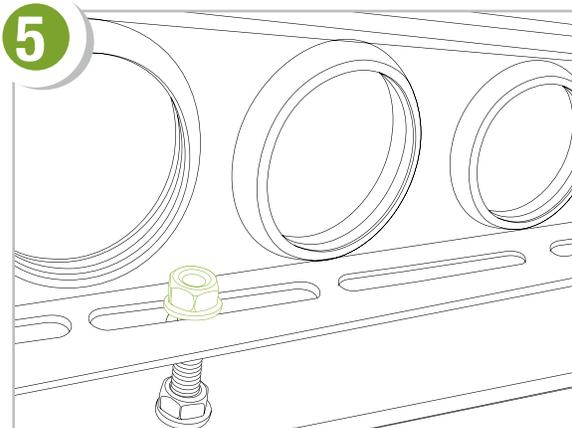
Insert the Stiebel Eltron S-Power high performance heatpipe tube into the rubber rings, which have to be lubricated beforehand with soap. **6**
