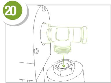
On the left hand side: lubricate the o-ring of the collector connection with silicone grease, connect the corrugated hose, push the side cap over the corrugated hose and mount. Following this pull the insulation over the hose. 21 + 22 + 23
