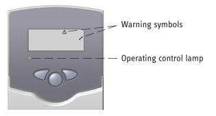
Operating control lamp flashes red. On the display the symbols  $\checkmark$  and  $\triangle$  appear.
