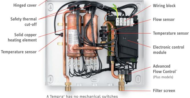
A Tempra<sup>®</sup> has no mechanical switches and is completely silent while operating.
