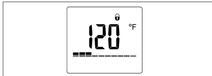
If the display-lock is active, a lock symbol will appear on the base display, and no parameters can be changed. In order to disable the lock, hold the  $T_{max}$  button for 12 seconds. The lock will disappear from the display and all parameters can be changed again.
