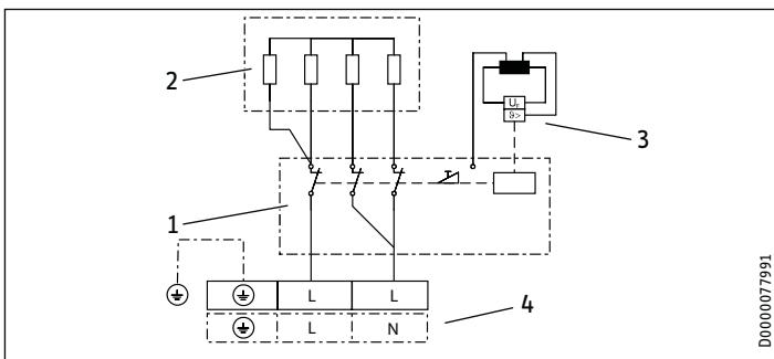
1 Power PCB with integral safety switch
