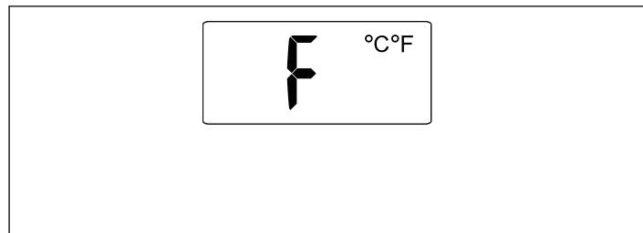
The current unit will be shown and the display will be flashing to indicate that the value can be changed. Rotate the control knob to change the value between Fahrenheit and Celsius.
