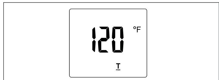
At the T<sub>max</sub> setting menu, the display will flash, indicating that the value can be changed by rotating the control knob. The T<sub>max</sub> value can be increased by turning the control knob clockwise, and decreased by turning it counter-clockwise. The T<sub>max</sub> value can be deactivated by turning the control knob counter-clockwise, past the 68 °F (20 °C) setting. The display will read "Off" if T<sub>max</sub> is inactive.
