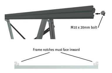
6. Position the mounting frames over the hypotenuse rail on the triangular racks. Insert the bolt through the hole in the hypotenuse rail. Loosely thread the nut onto the bolt on the inside of the U-Channel. Make sure the notches in the frames face inward.
