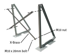
4. Use the M6 bolt and nut to secure the two X-Brace pieces together.
