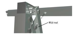
7. If multiple collectors are being installed, use the frame connector kit to fasten two frame pieces together. Slide the bolts into the groove on the short side of the frame piece. Abut the two frames together, and tighten the bolts over the frame connector.
