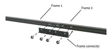
8. Before the assembly is bolted to the roof mount, the bolts for the collector fastening clips must be slid into the short side slot of all mounting frames. Slide four M10 x 20mm bolts in the short side of the mounting frame.Loosely attach the fastening clips to the bolts and lift them over the lip as shown for easy collector mounting.
