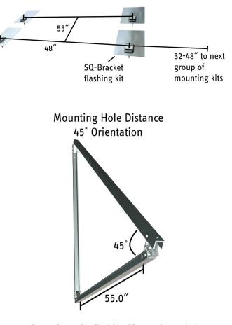
2. Fasten the racks to the flashing kits as shown below.
