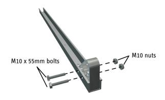
4. Repeat the process with the other M-103  $65^{''}$  rail using two more M10 nuts & bolts.
