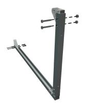
6. Complete the rack assembly by attaching t he remaining, M-102 92<sup>"</sup> rail and fastening it with two M10 nuts & bolts.
