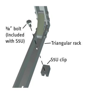
2. Clip the S5U assembly to the roof ridges.
