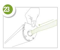
Screw on the connections, pull tight with a spanner and push the insulation over the corrugated hose.
