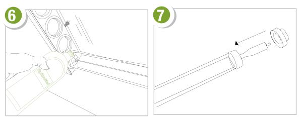
Place the safety rubber ring on top of the glass metal connection. 7 Rotate constantly the s-power high performance heat-pipe tube while inserting into the hole in the collector casing. 3 Insert the tube so the safety rubber of the heatpipe tube touches the end of the collector casing and then retrieve the tube out of the collector casing for 5mm. 9 Stiebel Eltron S-Power high performance heat pipe is now sealed.
