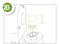
On the left hand side: lubricate the o-ring of the collector connection with silicone grease, connect the corrugated hose, push the side cap over the corrugated hose and mount. Following this pull the insulation over the hose. 21 + 22 + 33
