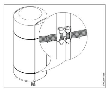
Ensure that the closures are positioned in the joint between a side insulation segment and the thermal insulation of the tank.
