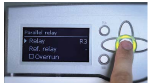
The SOM 10 features a full graphic display capable of showing historical sensor data and multiple sensors and relay values at once.
